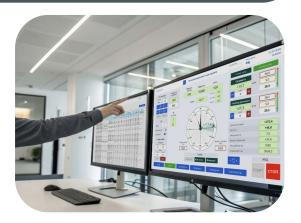
**RIGINTEL**, a Skolkovo resident based in Perm, offers an integrated digital suite for drilling control and optimization. It includes IR-Assistant (real-time monitoring), IR-Master (automated slide drilling), IR-OperBot+ (operator task automation), and IR-Vision (live video analytics). The ecosystem speeds up drilling, improves safety, ensures process precision, and reduces human error.
