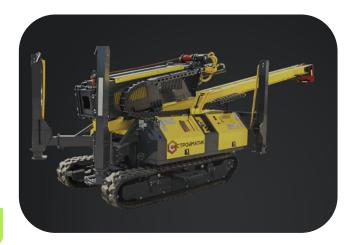
The Stroimatic pile driver is an innovative, compact crawler-mounted foundation machine designed for rapid and year-round piling in challenging and remote areas. Weighing between 2 and 5.5 tons, these machines enable one-day foundation installation, cutting construction time by up to 10× and costs by up to 2×. Easily transportable by trailer, boat, or helicopter, the product operates in all weather and terrain conditions.
