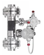
**Qualitet System** offers a cutting-edge multiphase flowmeter that enables accurate, real-time measurement of oil, water, and gas within a single pipeline. The device is capable of operating across a broad range of flow conditions, including high gas or water cut. It is suitable for individual wellheads, group metering units, test separators, and challenging operational environments.
