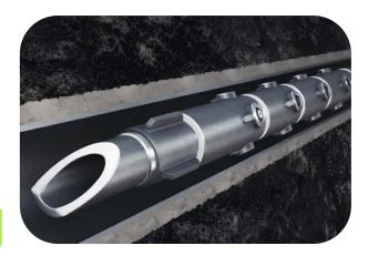
**OilTec** provides a high-tech solution for non-explosive perforation of wells using hydro-slotted perforators, followed by hydraulic fracturing and acidizing—all in a single trip by the well workover team. This method eliminates explosives, preserves casing integrity, and allows multiple perforations in one run while streamlining stimulation, resulting in significant time savings, enhanced safety, and improved well productivity.
