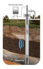
**Tri-Logic**, a Skolkovo resident since 2016, develops wireless Industrial IoT telemetry systems for the oil & gas sector. Their LoRaWAN-based surface networks collect real-time well data without cabling, while the wireless downhole system Tri-Logic.DCS transmits subsurface data intact. Deployed in Tatarstan and Orenburg, with clients including Tatneft and RuslanOil, the DCS system is now in successful pilot testing at Tatneft sites.
